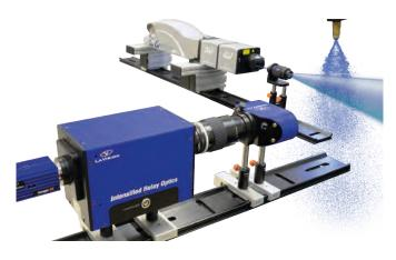
Laser Induced Exciplex Fluorescence (LIEF) allows simultaneous visualization of the two phases. Due to the special LIF tracers the signals from the liquid and the vapor phase can be spectrally separated by optical filters.
