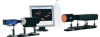
Based on imaging shadow projections of droplets the method of Shadowgraphy is applied in a small volume at a desired position within a spray (local). Quantitative absolute results are obtained and a range of lightsources from pulsed LEDs to lasers can be used as backlight source. A long distance microscope assures a safe working distance at a high magnification to even detect very small droplets.
